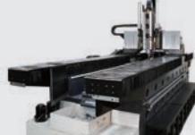
XYZ stage for laser marking and precision parts assembly
