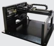
H-drive gantry stage for assembly and testing
